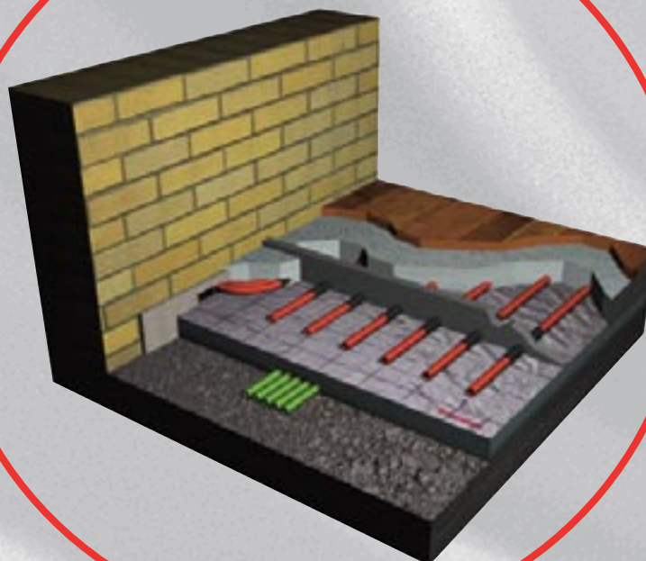
FLOOR EXPANSION JOINT
